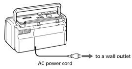
**For critical recording,** operating the player on AC power is recommended.
